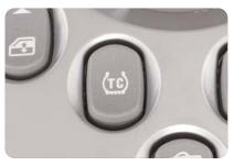
When off, the Traction Control System's "OFF" telltale light will illuminate and remain on. Turn the system back on at any time by pressing the button again. The system will default to ON when the ignition is cycled.
